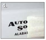
To expose product, pull pre-masking away at an angle as shown above, using a continuous motion. If bubbles occur in the letters, simply prick with a needle and smooth. Do not use a knife or razor
