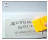
Apply pressure-sensitive vinyl to prepared surface, then squeegee pre-mask surface using overlapping strokes.
